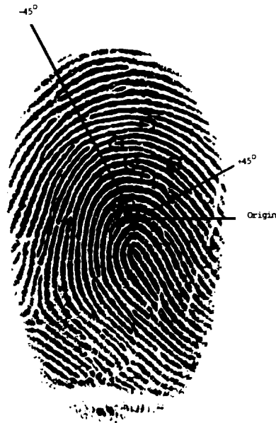
FIG. 4—Selection of neighbor minutiae. Neighbor minutiae are selected with ridge counts ranging from N6 to P9 within a 90° sector centered on the focal minutia.
