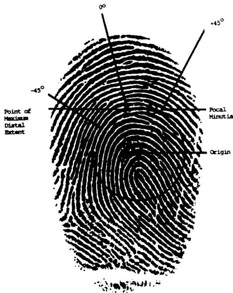
FIG. 3—Selection of the focal minutia. The focal minutia is selected from within a 90° sector centered where the ridges are at maximum curvature. If no minutia is found on the 5-mm ridge, successively more distal ridges are searched until a focal minutia is found.
